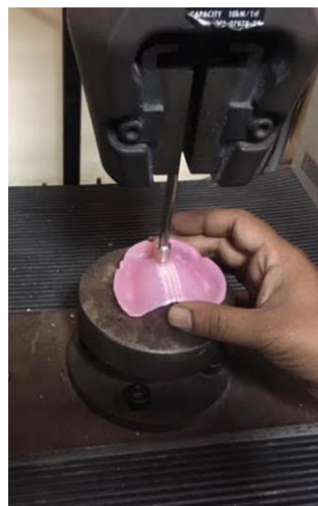
Fig 5: testing the partially reinforced denture using the Universal testing machine
