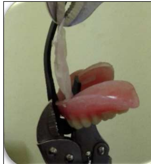
Fig 3: Peel bond strength test of the denture by using the universal testing machine
