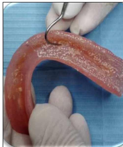
Fig 4: Using a fine probe for determining the type of failure (cohesive or adhesive).
