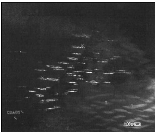
Fig 6: Transformation zone in thin foil of toughened ceramic.
