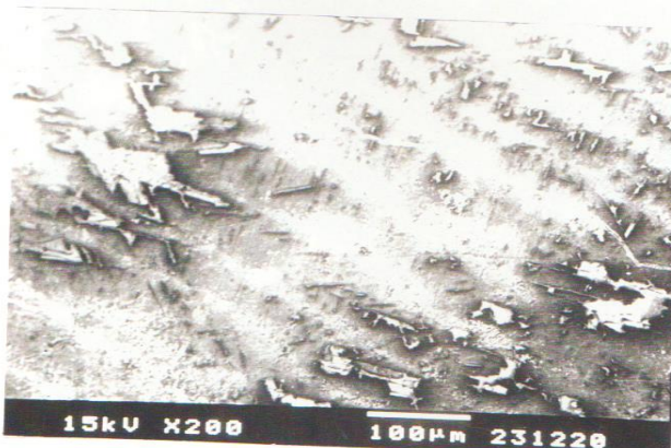
Fig 2: Scanning Electron Microscopic Picture of Acidulated Phosphate Fluoride Application After Acid Etching
