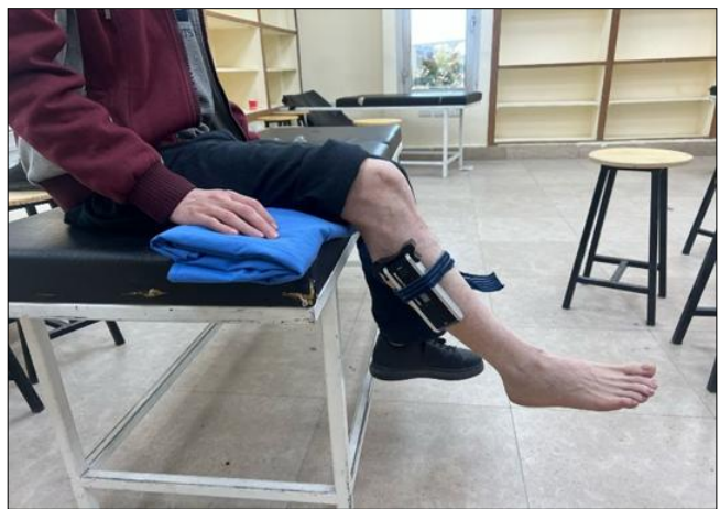
Fig 4: Target angle of 30° from the initial position (90° knee flexion)
